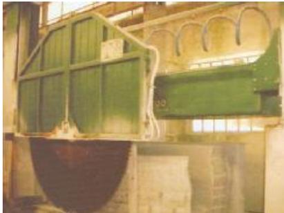
We had a case of an exclusive material that we bought from the quarry owner for two of our American distributors, but the quality of production wasn't right. He was cutting the blocks into slabs one at a time with a single bladed block cutter (see photo at left). There are uses for this machine, but not for producing gauged 3cm slabs.
